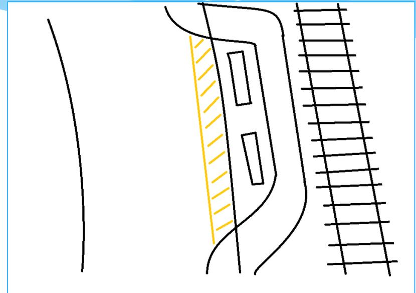
From a PBOT Traffic Engineering Report from Mark Haines (3/25/2014): “[...] Bridge columns narrowed the pavement width by approximately two feet for a length of approximately 70 feet. That width was taken entirely out of the bike lane [...] I recommend referring the request to a CIP list for future consideration.”
